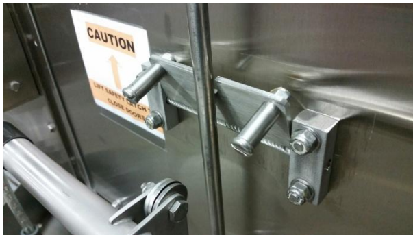
To lift the door, pull the arm upward
