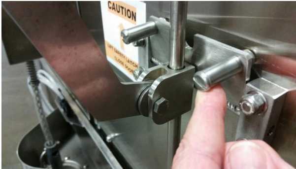
Continue to pull the arm down until the slider reaches the bottom of the rod.
