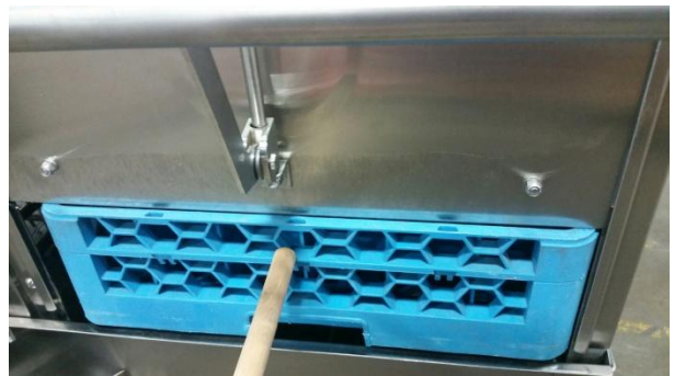
Pushing the rack with the hand allows the door to drop
