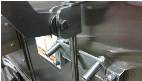
Slider moves above the latch plate
