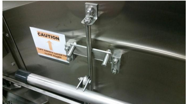
Continue to pull the arm down until the slider reaches the bottom of the rod.
