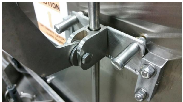
The slider will move passed the latch plate
