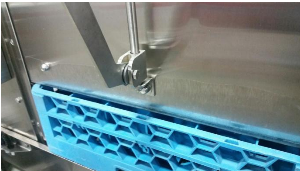
Rack is not pushed all the way into the machine
