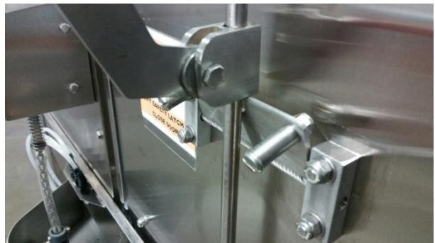
Pulling the door handle down, stops on the latch
