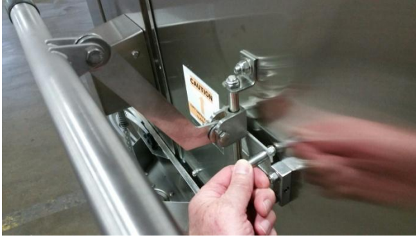
To pull the handle down fully, lift the safety latch up
